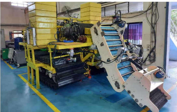
The deep-sea mining machine at the National Institute of Ocean Technology office in Chennai. This machine will move on the seafloor, collecting the nodules along with some soil, a quantity of around 40-50 kilograms per second. Photo from NIOT.
